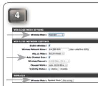
Select the Wi-Fi network (SSID) you want to extend/repeat from the list. If the Wi-Fi network requires a password, enter it in the **Pre-Shared Key** box above.
